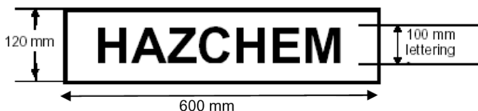
Figure 13.1 Form and dimensions of outer warning placard
